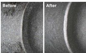
Removes the burrs at the edges that occurred during the manufacturing process, and round the end faces to prolong tool life.
